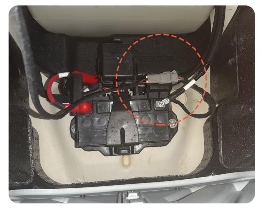
Locate the diagnostic connector, remove the white blank cover and connect Ototrak (picture above).
